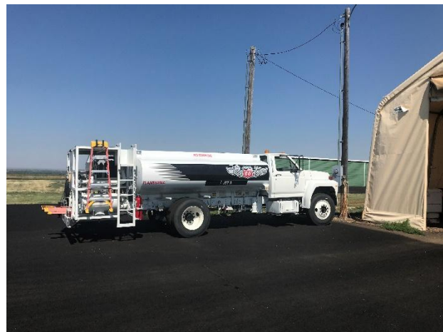
Figure 1-13. Jet A Fuel Truck
